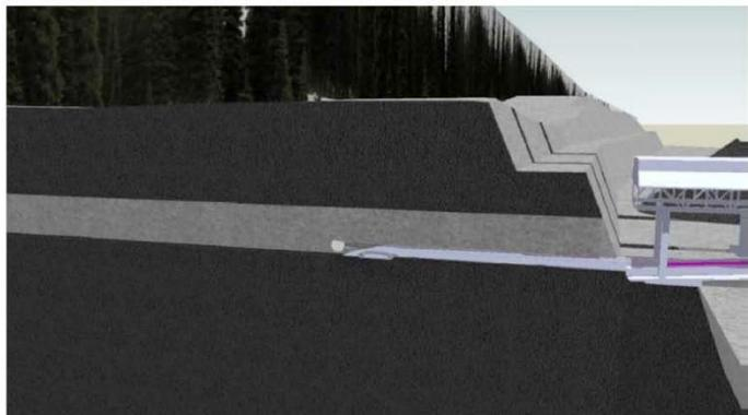
3. Profile of ADDCAR unit retreating from mined entry. Note pillar of coal above mined out entry.
