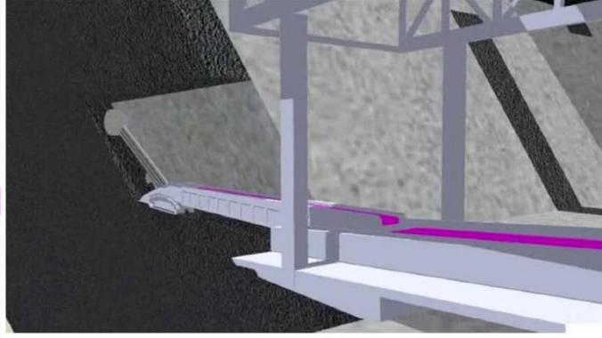
2. ADDCAR Highwall mining system penetrating steeply dipping seam
