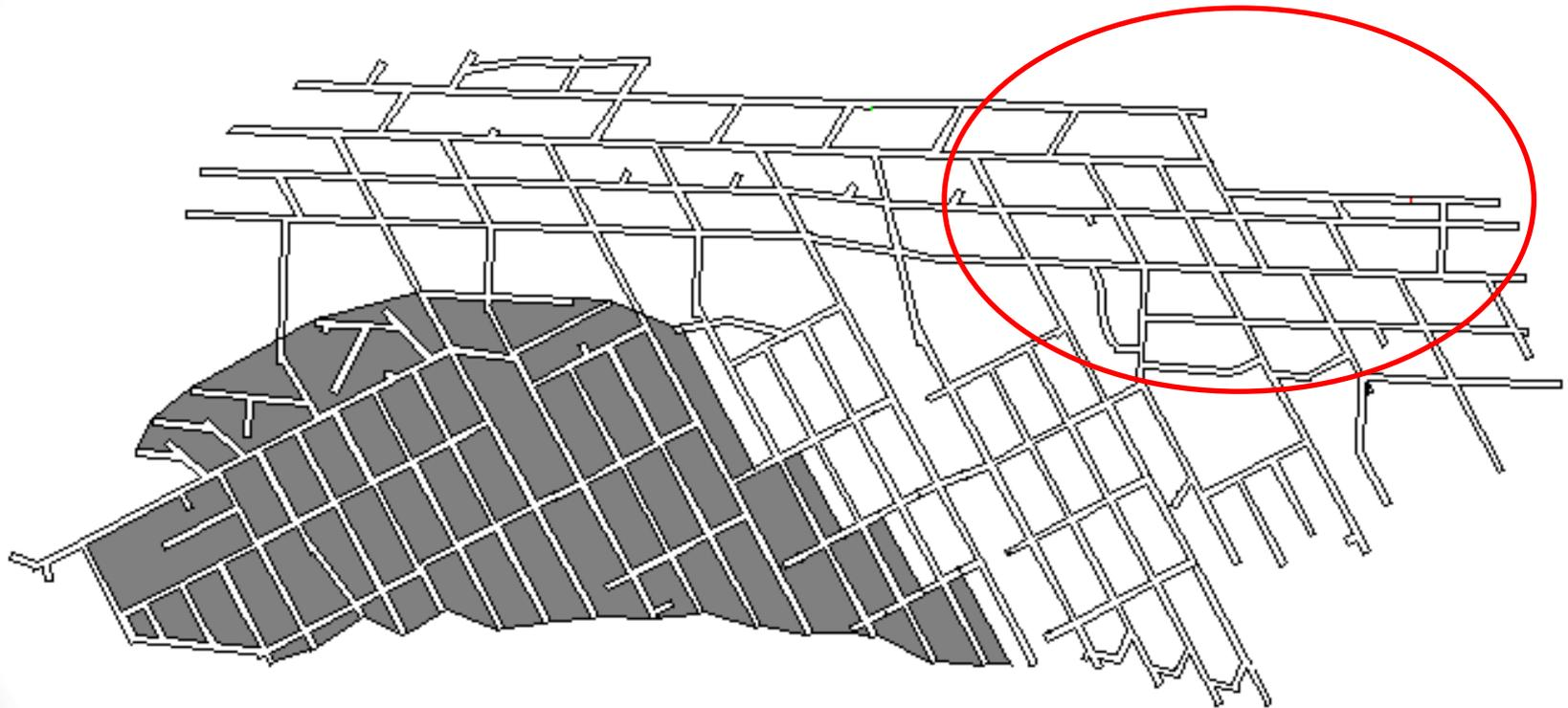
Structural blocks still spring surprises – realignment of main entries due to thrusting
