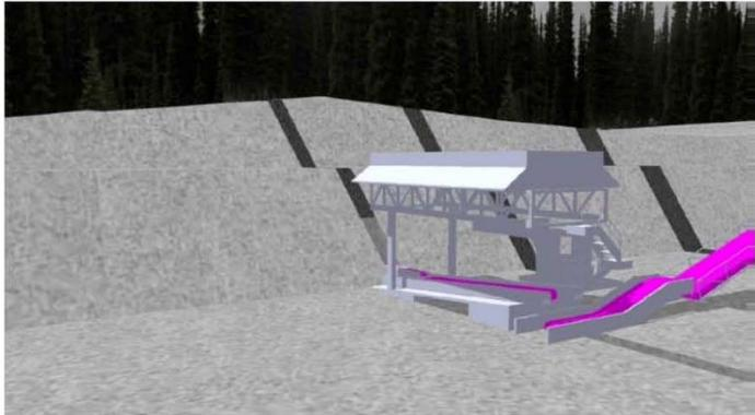
1. Launch vehicle positioned on mine bench in front of steeply dipping seam exposed in highwall
