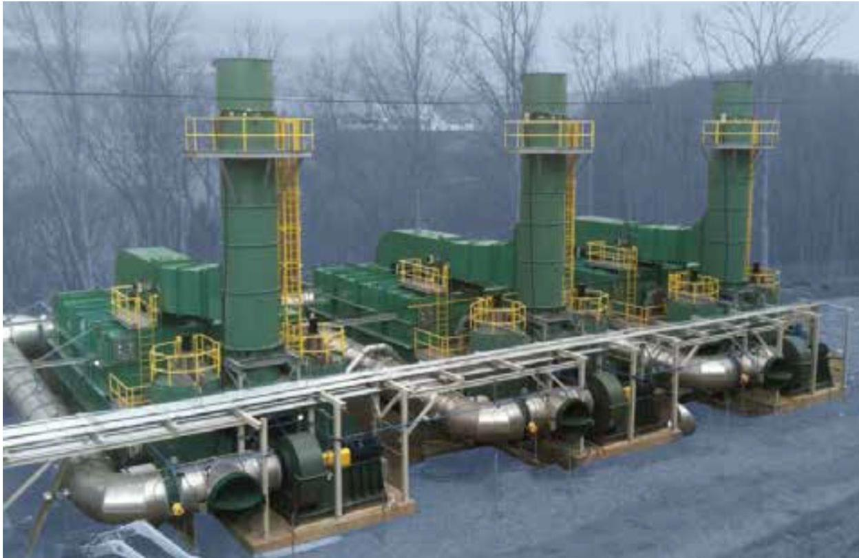
or conversion to heat and destruction: Ventilating air methane regenerative thermal oxidisers at McElroy Mine in the USA.
